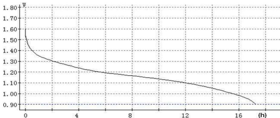
Test Condition: Load Resistor 3.9Ω, 24hrs/day, 20°C±2°C and 60±15%RH
