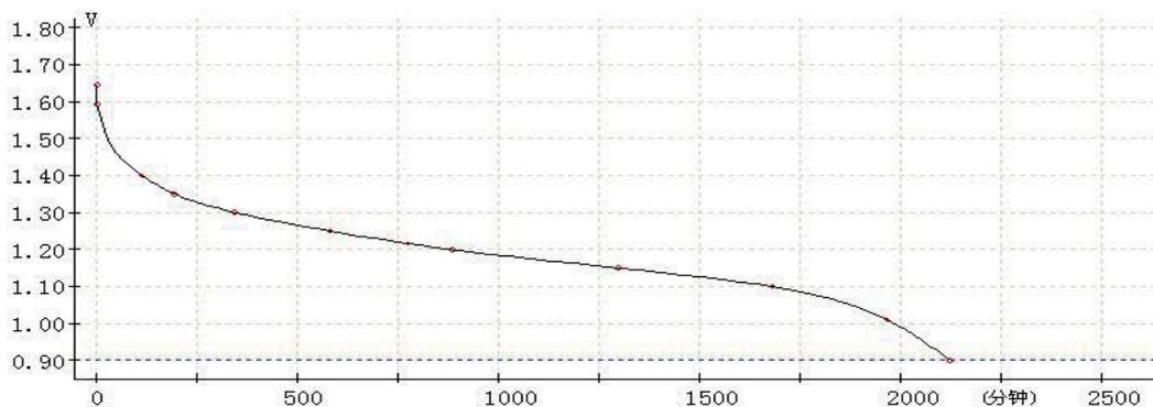
Test Condition: Load Resistor 3.9Ω, 24hrs/day, 20°C±2°C and 60±15%RH
